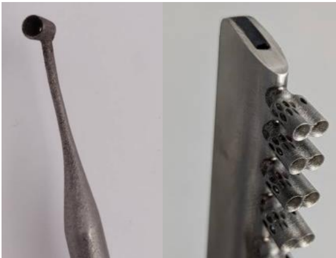
Figure 1: Kiel probe (left side) and rake with several Kiel probe heads installed (right side)
