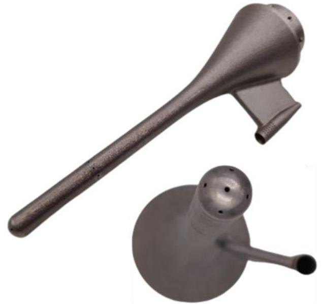
Figure 2: Air Data Boom head
