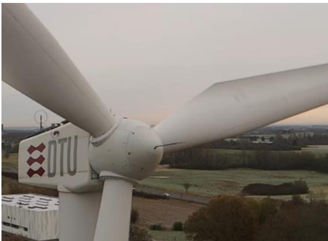
Figure 2: Picture of test turbine at DTU with Windflower system installed on the nose cone.
