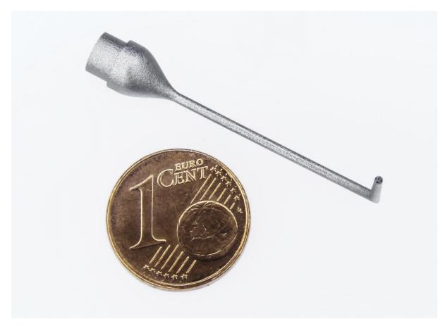
Abbildung 2 - Additively manufactured flow measurement probe from 3D MicroPrint
