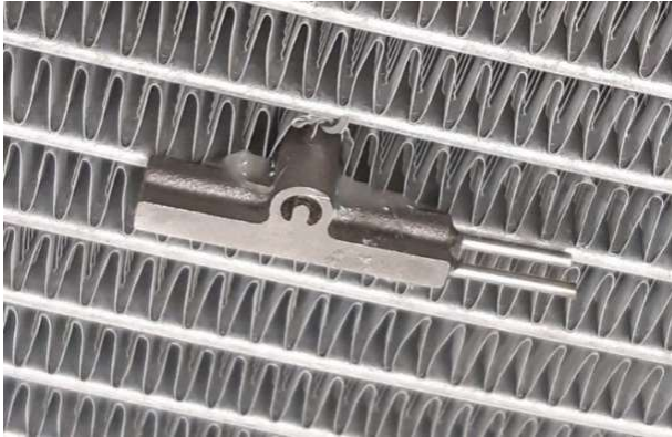
Figure 3 Probe (S_KPS_bujh36) mounted on radiator.
