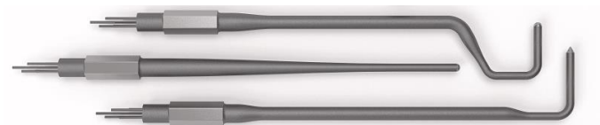
Figure 2: Shape examples (top to bottom: cobra probe, straight probe, L-shaped probe)
